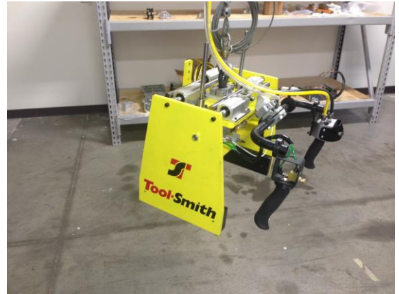
Clamping device actuated with pneumatic cylinders
