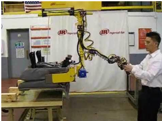
This device's adjustable center of gravity allows it to pick up different sized parts
