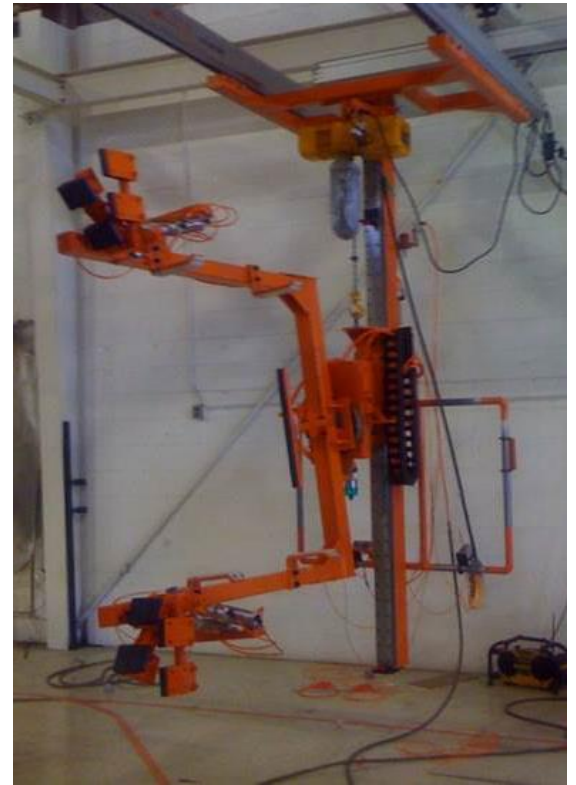
After this device lifts a watercraft, a motor rotates it 180 degrees
