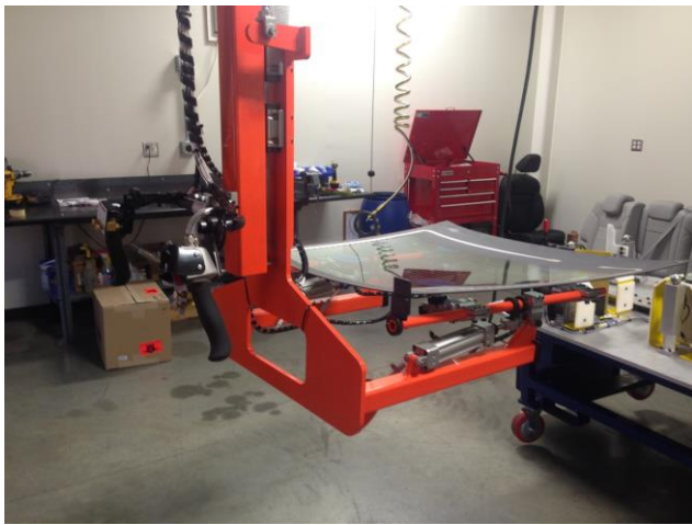
Cylinders tilt windshield 90 degrees into an upright position
