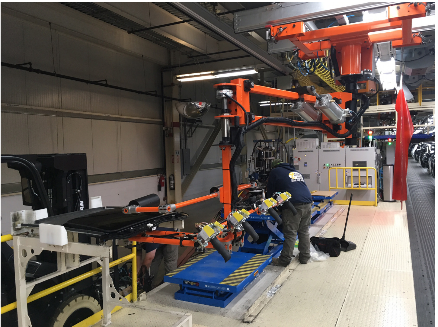
Rigid trolley and parallel link articulating arm add stability to this device
