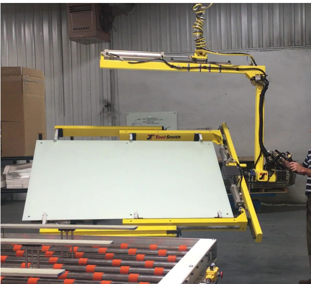
Pneumatic Oscillator- 180 Degree Glass Rotate Assist
