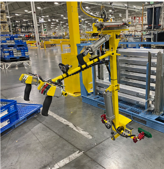
Cylinders tilt part upward 90 degrees, while weightless extended handles provide operator comfort
