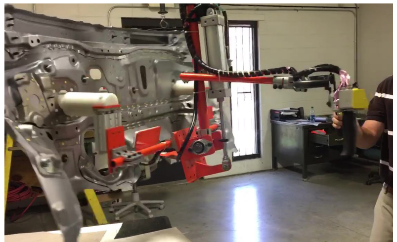
Cylinders tilt dashboard panel into an upright position
